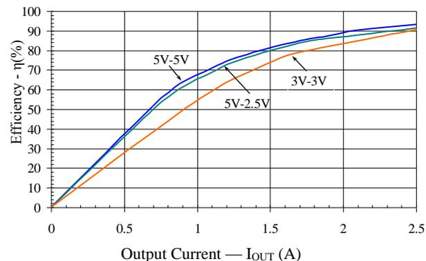
Figure 10. Efficiency vs.  $I_{OUT}$
