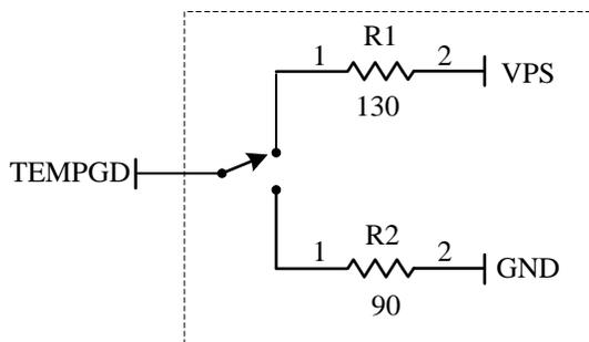
Figure 11. Internal Equivalent Circuit on  $TEMPGD$  Pin
