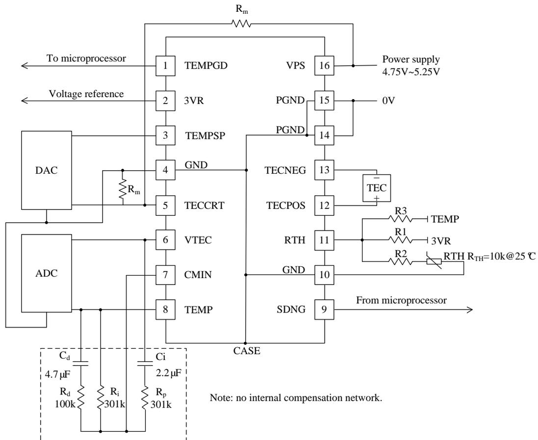
Figure 4. Microprocessor Based Application Circuit
