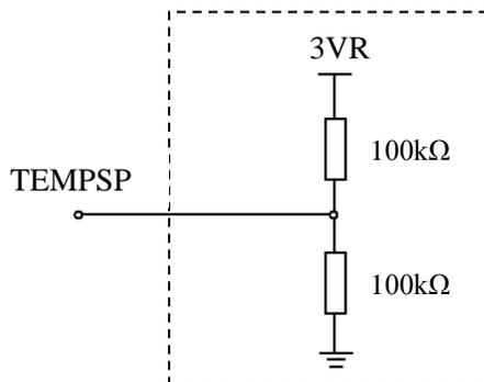
Figure 12. Internal Equivalent Circuit on TEMPSP Pin
