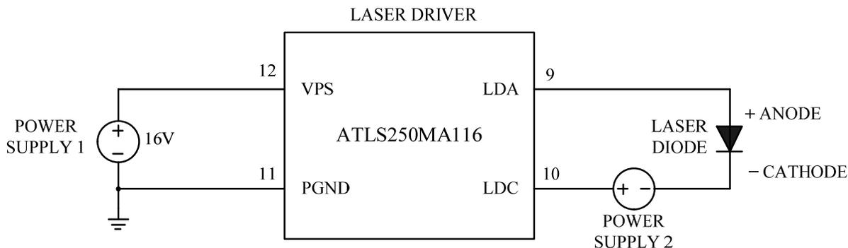
Figure 16. Driving High Voltage Laser Diodes
