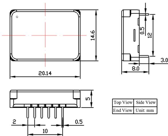
Figure 21. Dimensions of the DIP Package Controller
