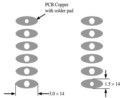
Figure 24. Top View of the Bottom Side PCB Foot-print
