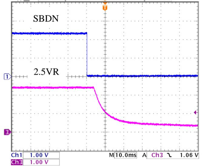
Figure 18. The fall time of SBDN vs. 2.5VR
