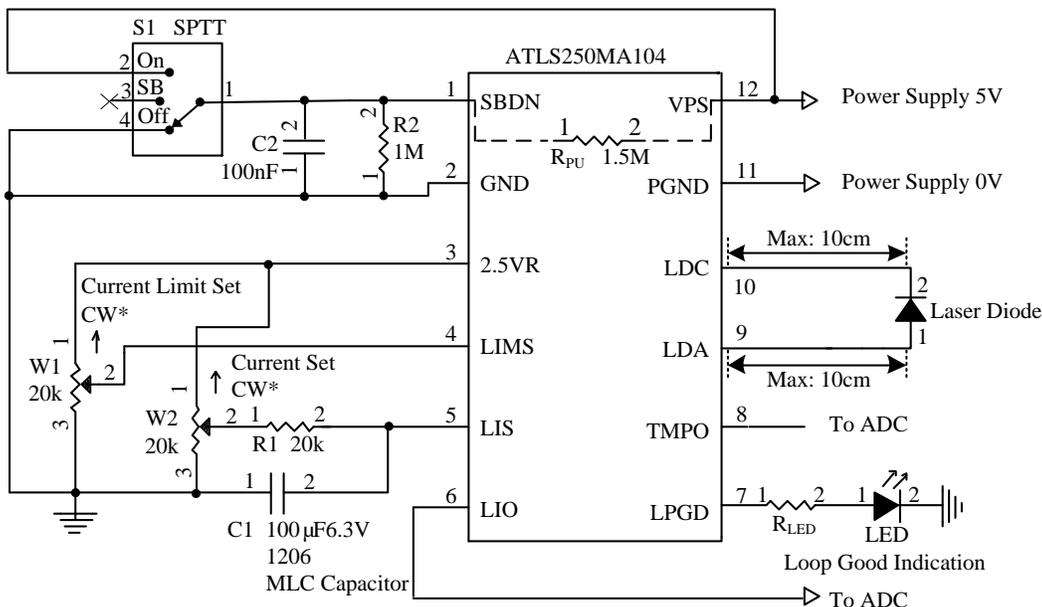
Figure 5.1. Typical Stand-alone CW Operation Schematic for ATLS250MA104
