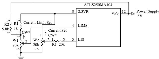
Figure 7.  $V_{LIMS}$  setting larger than  $V_{LIS}$
