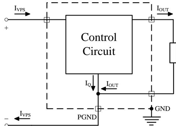
Figure 10. The Current Distributions in the Controller
