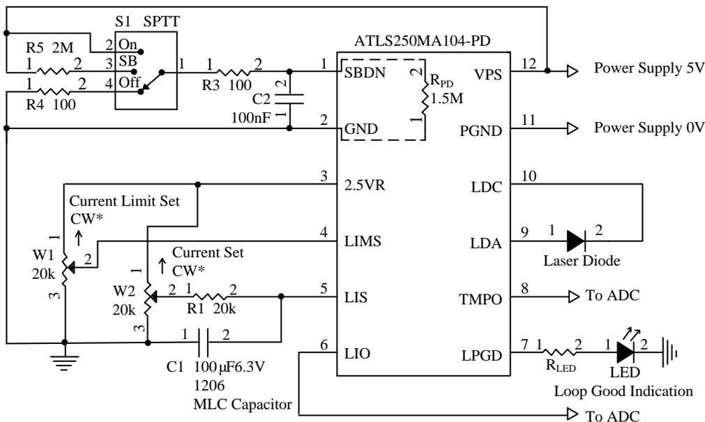
Figure 5.2. Typical Stand-alone CW Operation Schematic for ATLS250MA104-PD
