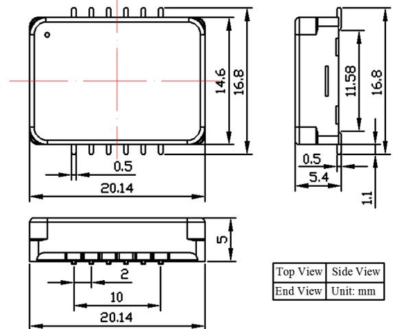
Figure 22. Dimensions of the SMT Package Controller
