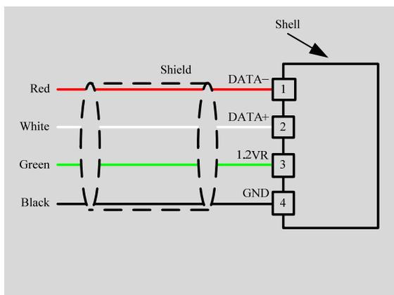
Figure 3. Connecting DAC Board to the Laser Driver ATLS1A118
