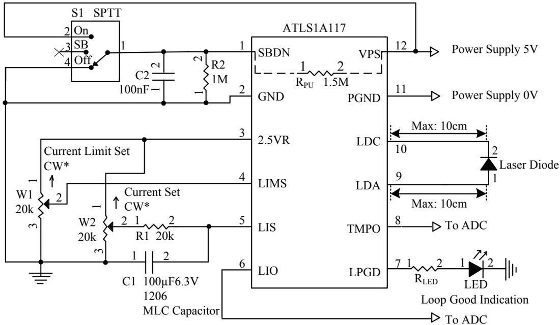
Figure 5.1. Typical Stand-alone CW Operation Schematic for ATLS1A117
