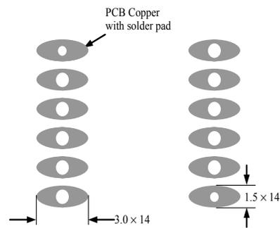
Figure 22. Top View of the Bottom Side PCB Foot-print
