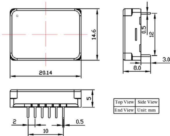
Figure 19. Dimensions of the DIP Package Controller
