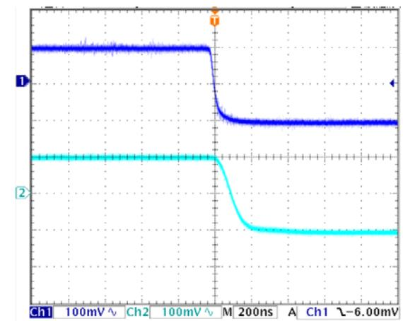
Figure 12.4. Small Signal Fall Time 200ns
