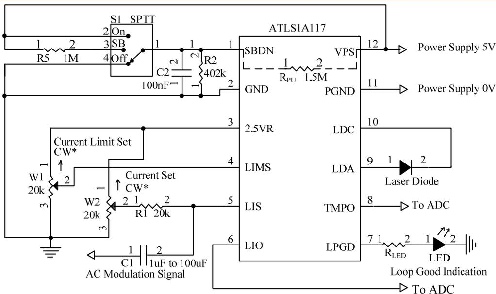
Figure 5.3. Typical AC Modulation with DC bias Schematic for ATLS1A117
