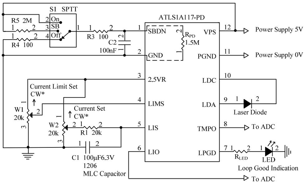
Figure 5.2. Typical Stand-alone CW Operation Schematic for ATLS1A117-PD
