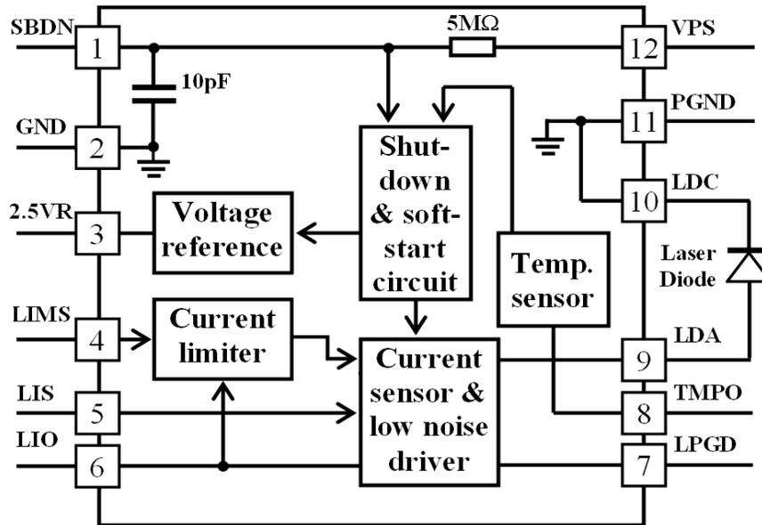
Figure 4. Block Diagram
