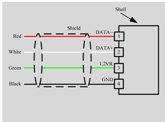
Figure 3. Connecting DAC Board to the laser Driver ATLS100MA118
