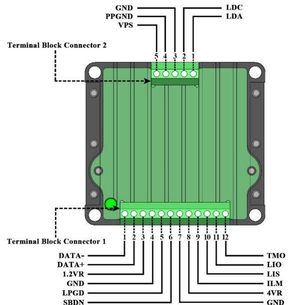
Figure 4. Top View of ATLS100MA118
