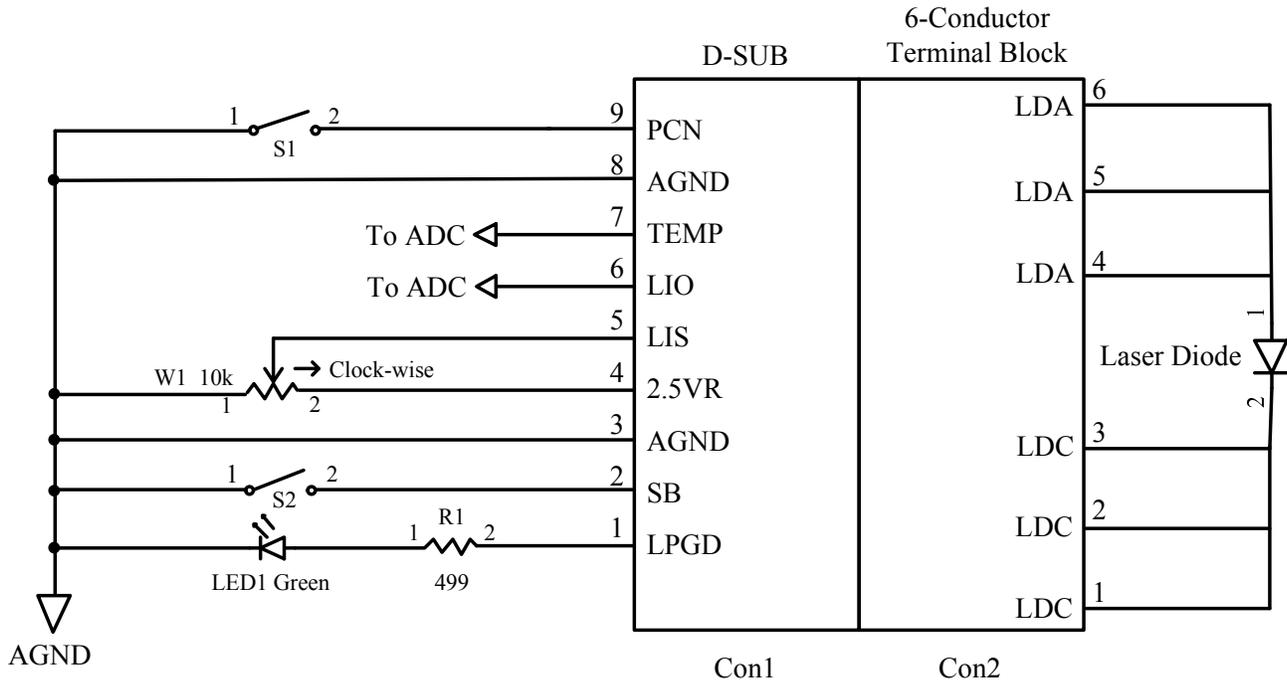
Figure 2. A Typical Application Schematic
