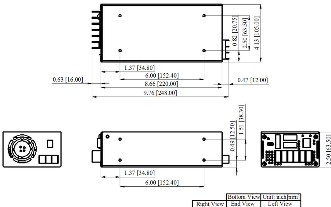
Figure 17. Mechanical Dimensions
