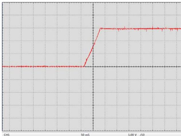
Figure 15. Start-up Waveform at LDA Pin
