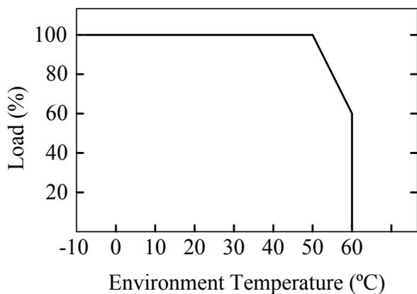
Figure 14. Derating Curve
