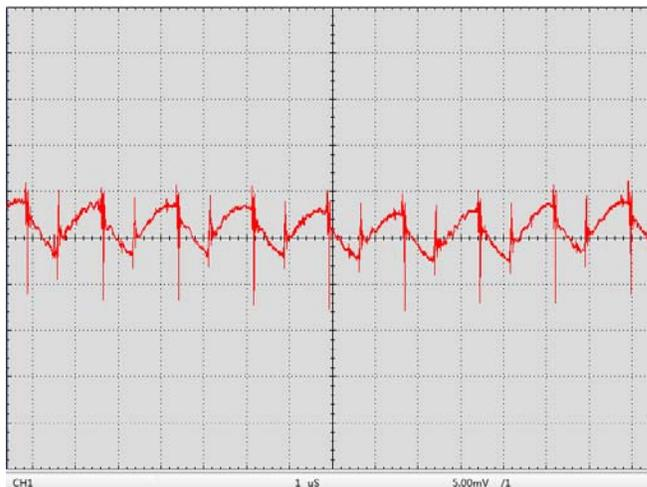
Figure 16. Noise Waveform at LDA Pin
